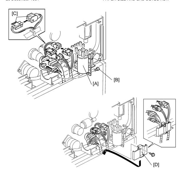
CAUTION: When closing the power supply section [A], use the grounding screw [B] (#6) for proper grounding.
