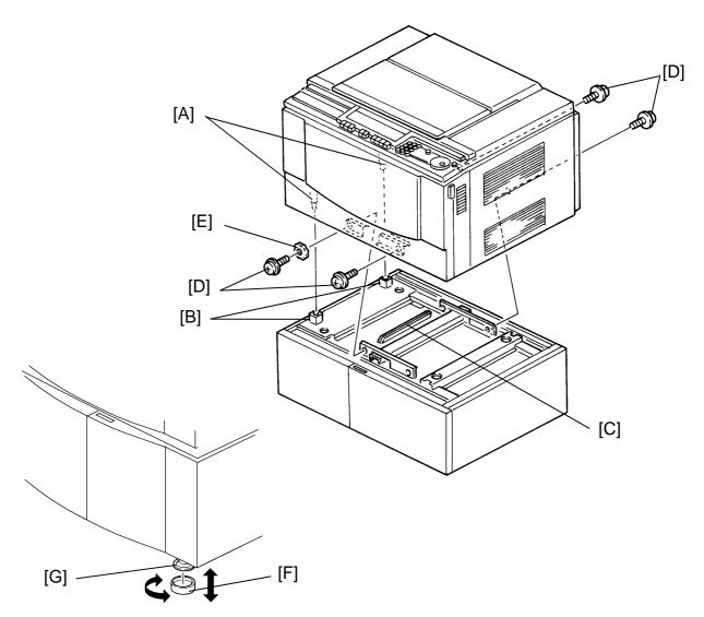
3. Place the copier on the paper feed unit aligning the positioning pins [A] of the copier with the positioning holes [B] of the paper feed unit.
